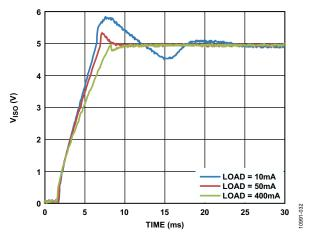
Figure 32. Typical V<sub>ISO</sub> Startup 5 V Input to 5 V Output with 10 mA, 50 mA, and 400 mA Output Load
