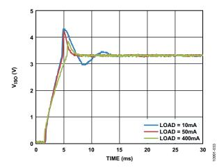
Figure 33. Typical V<sub>ISO</sub> Startup 5 V Input to 3.3 V Output with 10 mA, 50 mA, and 400 mA Output Load
