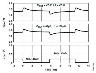
Figure 41. Typical  $V_{\rm ISO}$  Load Transient Response 3.3 V Input to 3.3 V Output at 10% to 90% of 250 mA Load at 500 kHz  $f_{\rm SW}$  with 0.1  $\mu$ F Feedback Capacitor
