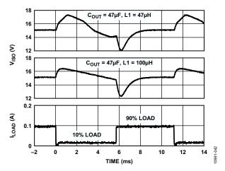
Figure 42. Typical  $V_{\rm ISO}$  Load Transient Response 5 V Input to 15 V Output at 10% to 90% of 100 mA Load at 500 kHz  $f_{\rm SW}$
