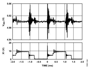
Figure 44. Typical  $V_{\rm ISO}$  Output Ripple, 5 V Input to 5 V Output at 400 mA Load at 500 kHz  $f_{\rm SW}$
