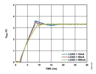
Figure 34. Typical  $V_{\rm ISO}$  Startup 3.3 V Input to 3.3 V Output with 10 mA, 50 mA, and 250 mA Output Load
