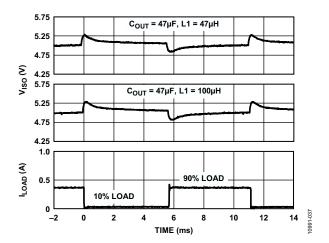
Figure 37. Typical  $V_{\rm ISO}$  Load Transient Response 5 V Input to 5 V Output at 10% to 90% of 400 mA Load at 500 kHz  $f_{\rm SW}$  with 0.1  $\mu F$  Feedback Capacitor
