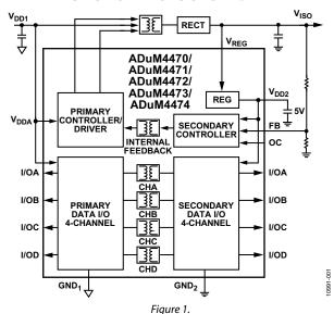
The regulated feedback provides a relatively flat efficiency curve over the full output power range. The ADuM447x enable a dcto-dc converter with a 3.3 V to 24 V isolated output voltage range from either a 5.0 V or a 3.3 V input voltage, with an output power of up to 2.5 W.
