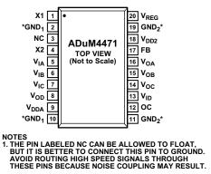
\*PIN 2 AND PIN 10 ARE INTERNALLY CONNECTED, AND CONNECTING BOTH TO GND<sub>1</sub> IS RECOMMENDED. PIN 11 AND PIN 19 ARE INTERNALLY CONNECTED, AND CONNECTING BOTH TO GND<sub>2</sub> IS RECOMMENDED.
