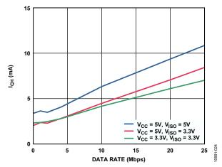
Figure 24. Typical Single-Supply I<sub>CH</sub> Supply Current per Forward Data Channel (15 pF Output Load)
