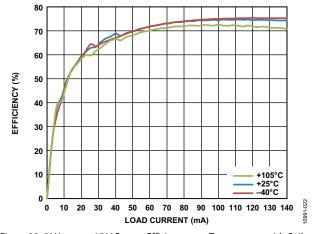
Figure 22. 5 V Input to 15 V Output Efficiency over Temperature with Coilcraft Transformer (CR7984-CL) at 500 kHz  $f_{\rm SW}$
