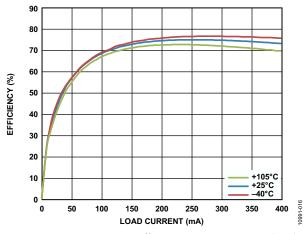
Figure 16. 5 V Input to 5 V Output Efficiency over Temperature with Coilcraft Transformer (CR7983-CL) at 500 kHz  $f_{\rm SW}$
