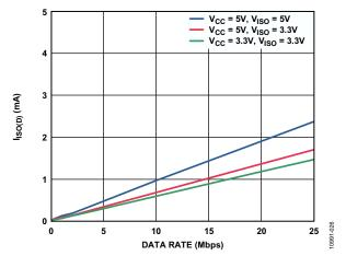
Figure 26. Typical Single-Supply I<sub>ISO(D)</sub> Dynamic Supply Current per Output Channel (15 pF Output Load)
