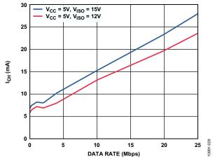
Figure 29. Typical Double-Supply I<sub>CH</sub> Supply Current per Reverse Data Channel (15 pF Output Data)
