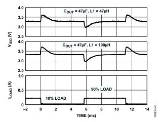
Figure 40. Typical  $V_{\rm ISO}$  Load Transient Response 3.3 V Input to 3.3 V Output at 10% to 90% of 250 mA Load at 500 kHz  $f_{\rm SW}$
