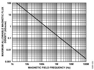
Figure 53. Maximum Allowable External Magnetic Flux Density
