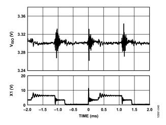
Figure 46. Typical V  $_{\rm ISO}$  Output Ripple, 3.3 V Input to 3.3 V Output at 250 mA Load at 500 kHz  $\rm f_{\rm SW}$
