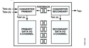
Figure 55. Power Consumption Within the ADuM447x
