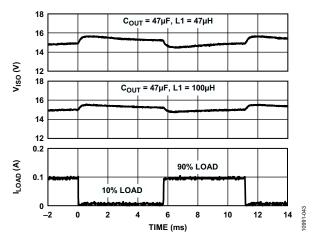
Figure 43. Typical  $V_{\rm ISO}$  Load Transient Response 5 V Input to 15 V Output at 10% to 90% of 100 mA Load at 500 kHz  $f_{\rm SW}$  with 0.1  $\mu F$  Feedback Capacitor
