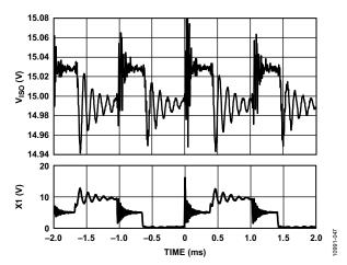
Figure 47. Typical V $_{\rm ISO}$  Output Ripple, 5 V Input to 15 V Output at 100 mA Load at 500 kHz  $f_{\rm SW}$
