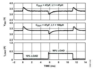
Figure 38. Typical  $V_{\rm ISO}$  Load Transient Response 5 V Input to 3.3 V Output at 10% to 90% of 400 mA Load at 500 kHz  $f_{\rm SW}$
