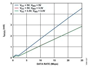
Figure 27. Typical Single-Supply  $I_{\rm ISO(D)}$  Dynamic Supply Current per Input Channel (15 pF Output Load)
