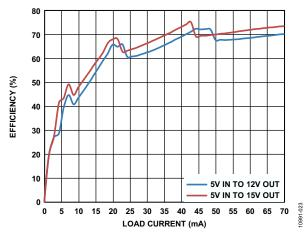
Figure 23. Double-Supply Efficiency with Coilcraft Transformer (CR7985-CL) at 500 kHz f<sub>SW</sub>
