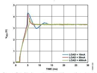
Figure 35. Typical V<sub>ISO</sub> Startup 5 V Input to 15 V Output with 10 mA, 20 mA, and 100 mA Output Load
