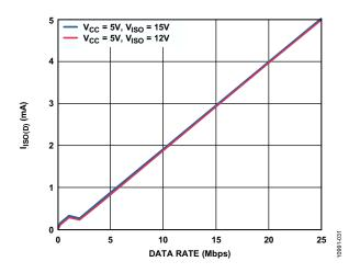
Figure 31. Typical Double-Supply I<sub>ISO(D)</sub> Dynamic Supply Current per Input Channel
