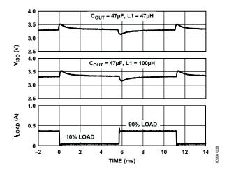
Figure 39. Typical V $_{\rm ISO}$  Load Transient Response 5 V Input to 3.3 V Output at 10% to 90% of 400 mA Load at 500 kHz  $f_{\rm SW}$  with 0.1  $\mu$ F Feedback Capacitor
