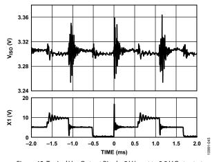
Figure 45. Typical  $V_{\rm ISO}$  Output Ripple, 5 V Input to 3.3 V Output at 400 mA Load at 500 kHz  $f_{\rm SW}$
