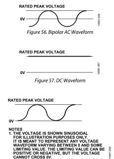
Figure 58. Unipolar AC Waveform
