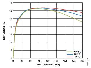
Figure 19. Typical Efficiency at 3.3 V In to 5 V Out over Temperature with 1:3 Coilcraft Transformer (CR7984-CL) at 500 kHz  $f_{\rm vw}$
