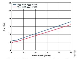
Figure 28. Typical Double-Supply Current I<sub>CH</sub> Per Forward Data Channel (15 pF Output Load)
