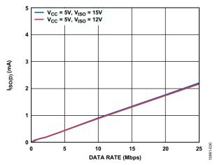
Figure 30. Typical Double-Supply  $I_{\rm ISO(D)}$  Dynamic Supply Current per Output Channel (15 pF Output Load)
