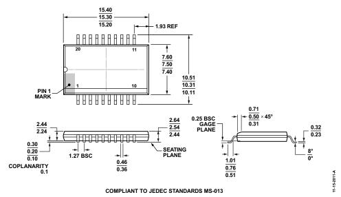
Figure 59. 20-Lead Standard Small Outline Package, with Increased Creepage [SOIC\_IC]
