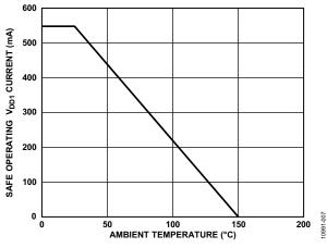
Figure 7. Thermal Derating Curve, Dependence of Safety Limiting Values on Case Temperature, per DIN V VDE V 0884-10
