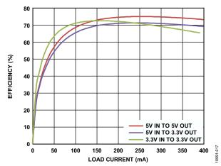
Figure 17. Single-Supply Efficiency with Coilcraft Transformer (CR7983-CL) at 500 kHz  $f_{\scriptscriptstyle \mathrm{SW}}$
