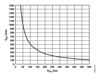
Figure 13. Switching Frequency ( $f_{SW}$ ) vs.  $R_{OC}$  Resistance
